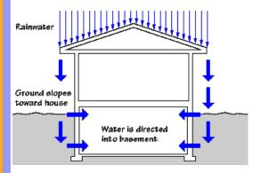
**PROBLEM:** If the ground around a foundation is level or slopes toward the house, water is directed into the basement. The soil next to the house is often backfilled without proper compaction and later settles. This is especially true under stoops where water can collect next to the basement wall.
