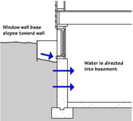
**PROBLEM:** Window wells are like a drain right next to the basement wall. Often they are improperly built so that any water is directed toward, rather than away from the foundation.
