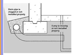
PROBLEM: Many existing houses simply have no subsurface drainage system. This comes from a time when basements were not used as habitable space. In other cases, the systems do not work for a variety of reasons, such as collapse of the pipe, clogging of the pipe with silt and/or tree roots, or a broken connection to the sump. The sump pit usually contains a pump designed to lift the water to the ground surface outside the foundation wall. This pump can fail.
