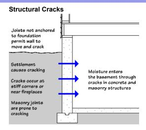
**PROBLEM:** Concrete and concrete block foundations usually develop some cracks. They can be severe if floor joists are not properly connected to the foundation wall, thus permitting the wall to move. Also, soil settling causes cracking. Places where walls meet rigid structures like the fireplace often crack as well. Usually, drainage removes the water from cracks, but repair may be necessary.
