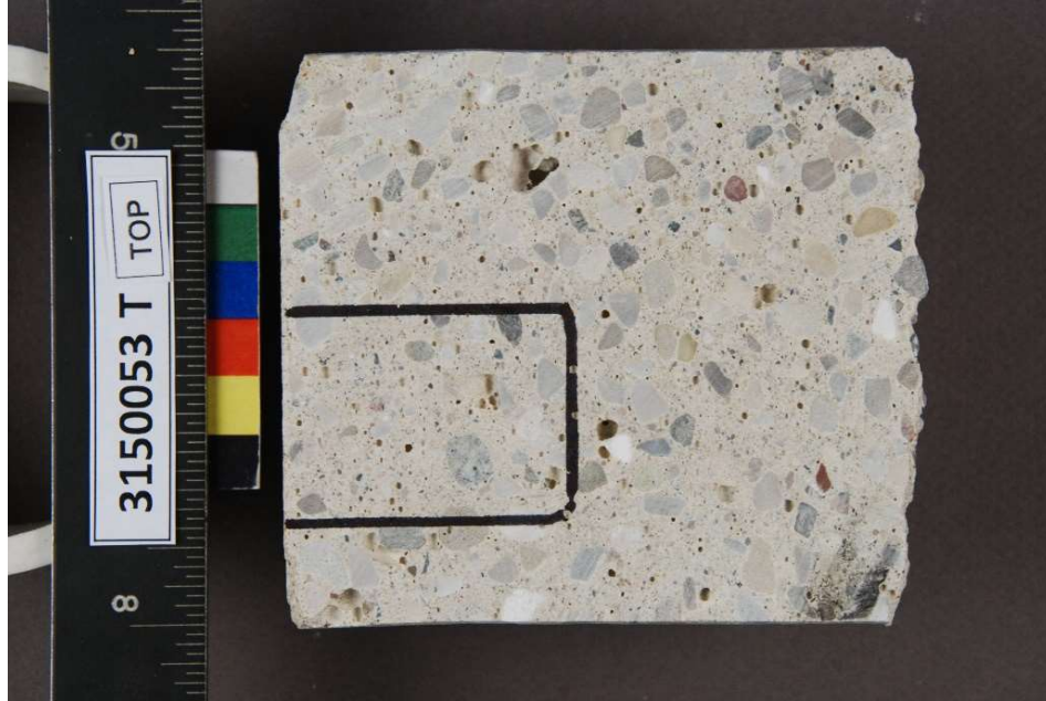
Figure 19. Pre-Cast Panel (3150053). Photograph of cross sectioned slab showing location of thin section preparation.
