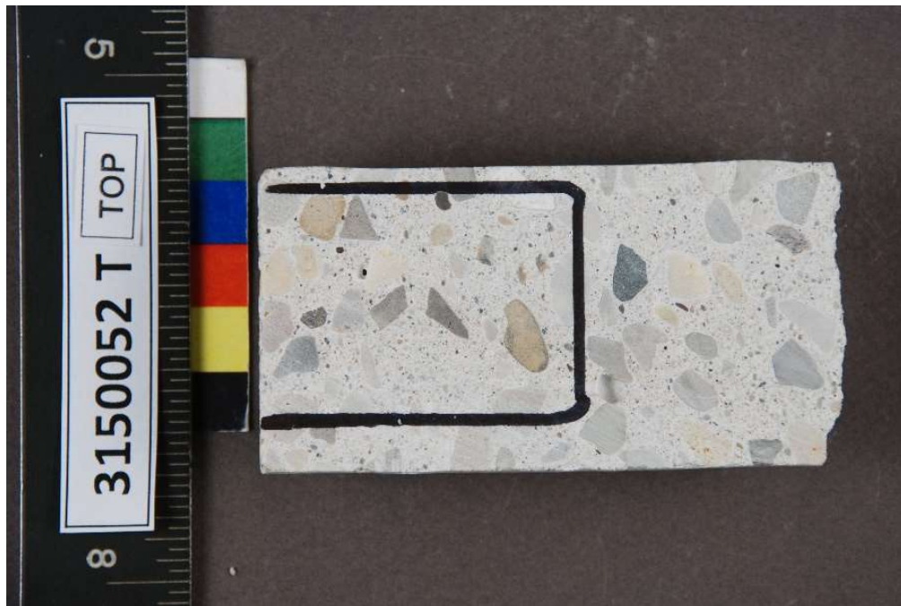
Figure 7. Fin (3150052). Photograph of cross sectioned slab showing location of thin section preparation.
