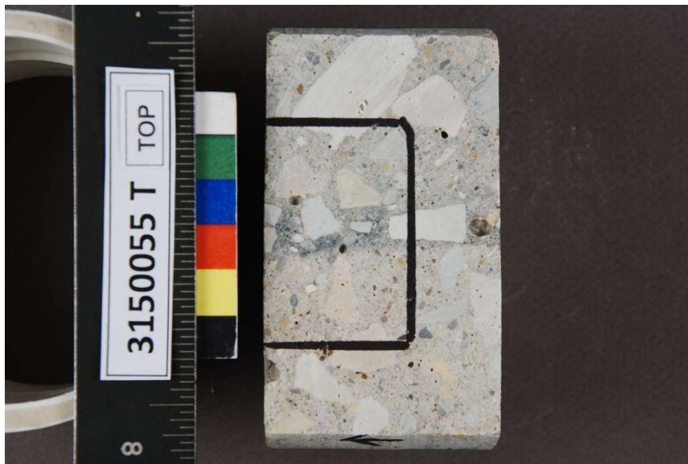
Figure 40. Entrance Wall (3150055). Photograph of cross sectioned slab showing location of thin section preparation.
