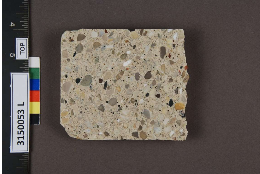
Figure 17. Pre-Cast Panel (3150053). Photograph of polished cross sectioned slab.
