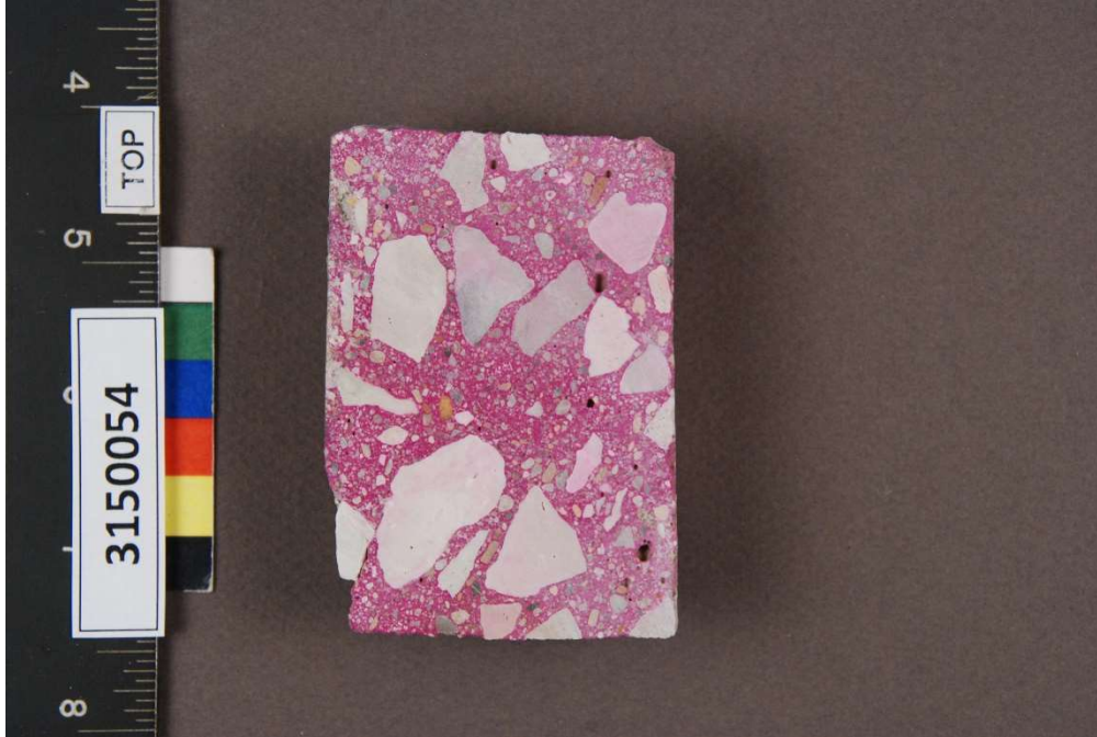
Figure 26. Column (3150054). Photograph of freshly cut surface with phenolphthalein indicator applied.
