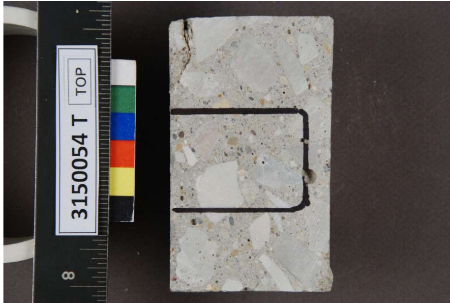
Figure 30. Column (3150054). Photograph of cross sectioned slab showing location of thin section preparation.
