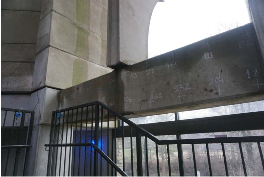
FIGURE 13 EMBEDDED TEMPERATURE HUMIDITY LOCATIONS
