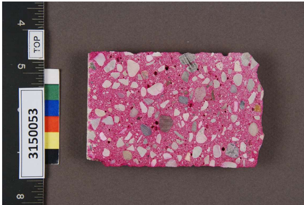
Figure 16. Pre-Cast Panel (3150053). Photograph of freshly cut surface with phenolphthalein indicator applied.
