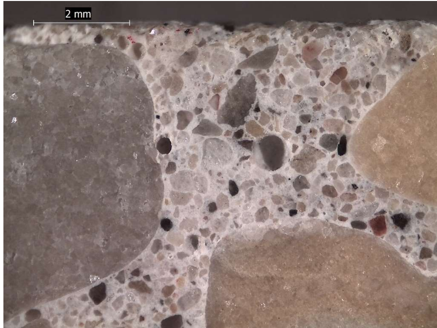
Figure 6. Fin (3150052). Stereo-optical micrograph showing exposed coarse and fine aggregates on the surface.
