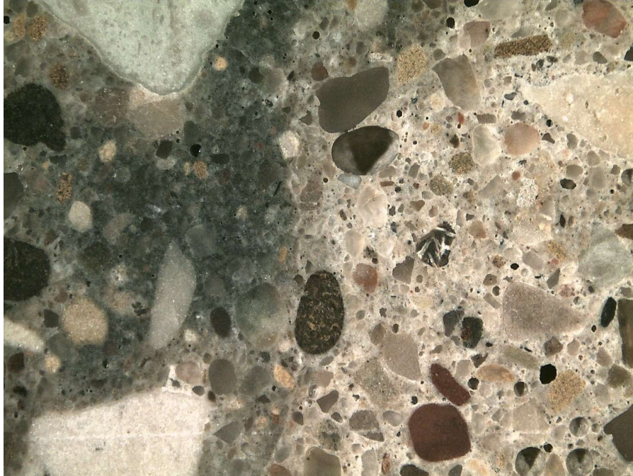
Figure 39. Entrance Wall (3150055). Stereo-optical micrograph showing the interface between concrete pours.
