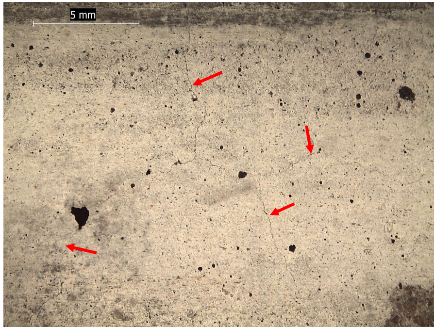
Figure 27. Column (3150054). Stereo-optical micrograph of the core side showing microcracks up to \frac{13}{16} " deep.
