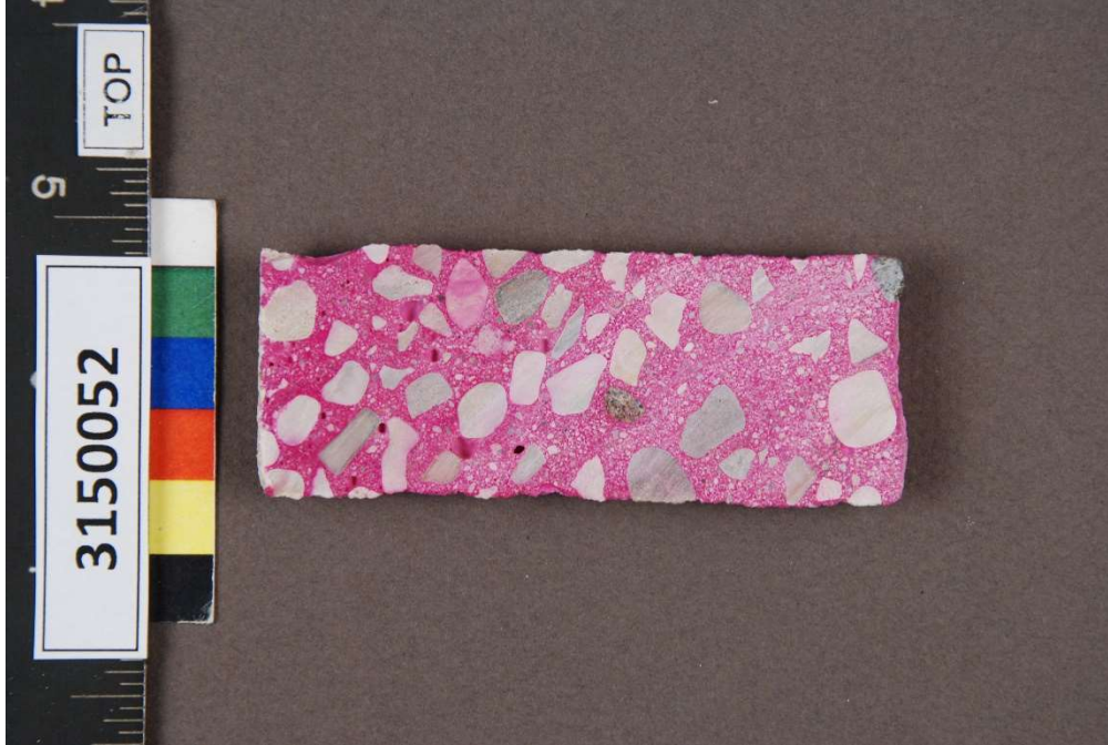
Figure 4. Fin (3150052). Photograph of freshly cut surface with phenolphthalein indicator applied.
