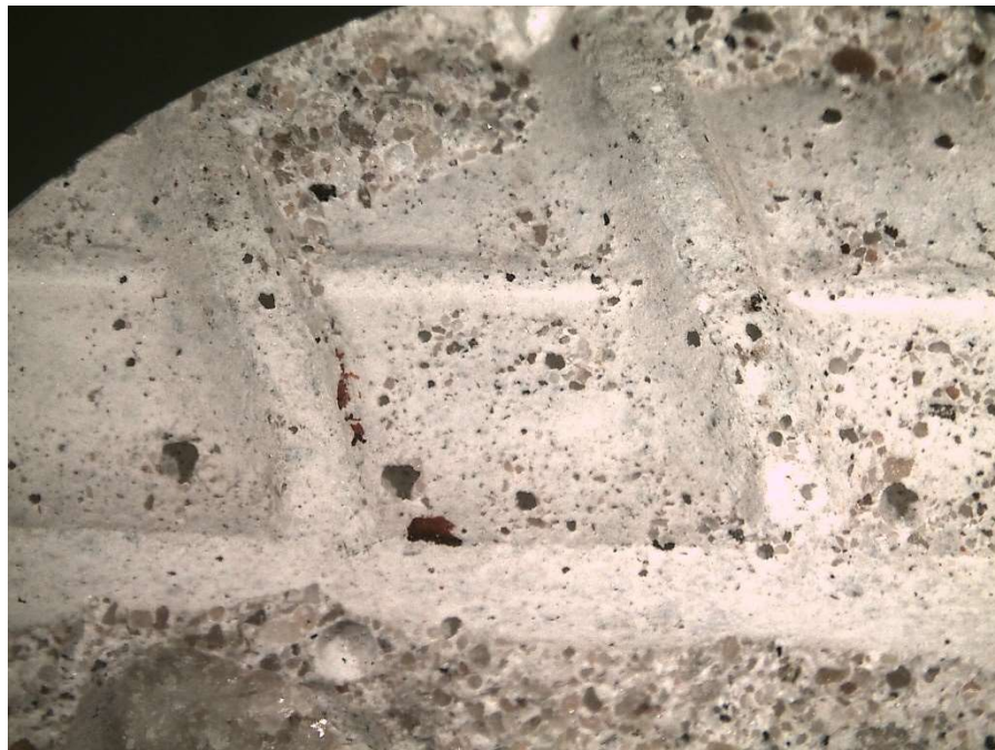
Figure 3. Fin (3150052). Stereo-optical micrograph showing the impression of the steel bar on the bottom of the core.
