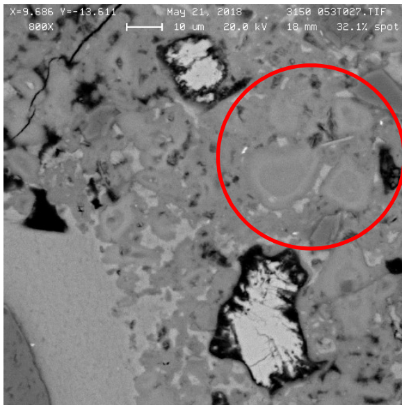
Figure 23. Pre-Cast Panel (3150053). BSE image showing two toned rims of hydrated Portland cement grains.
