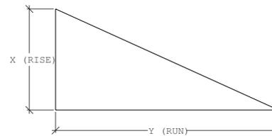
The rise over run diagram is used to determine the roof slope/pitch.
