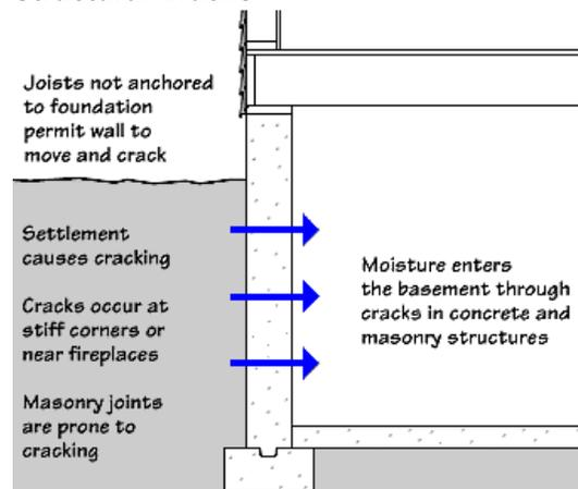
**PROBLEM:** Concrete and concrete block foundations usually develop some cracks. They can be severe if floor joists are not properly connected to the foundation wall, thus permitting the wall to move. Also, soil settling causes cracking. Places where walls meet rigid structures like the fireplace often crack as well. Usually, drainage removes the water from cracks, but repair may be necessary.
