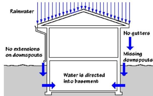
**PROBLEM:** Missing gutters and downspouts cause rainwater to be directed toward the foundation perimeter. Also, a downspout without an extender or splashblock is worse than no downspout at all. It is depositing the huge volume of rainwater from the roof in a single concentrated location near the basement.
