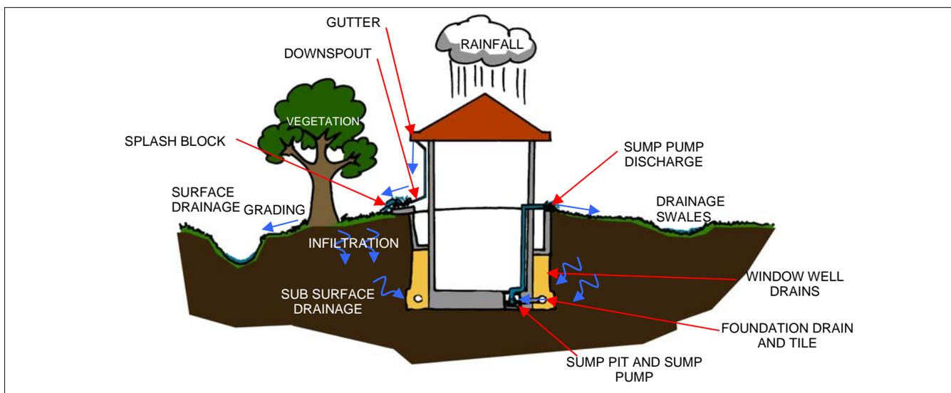
Protecting a home and its contents from damage due to surface water runoff and groundwater is a major concern for many homeowners. A properly designed, installed and maintained drainage system can provide this protection.
